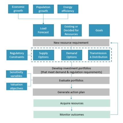
Figure 2. Generalized Capacity Expansion Planning Schematic
