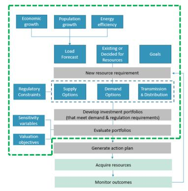
Figure 3. Aspects Addressed by Capacity Expansion Models
